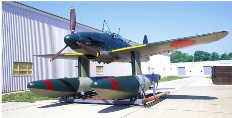
a collapsible catapult carriage, attach the plane's floats and have it readied for flight in approximately 7 minutes.
