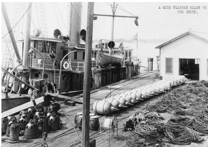
Mine planter at a dock, ready to load mines and associated equipment 34
